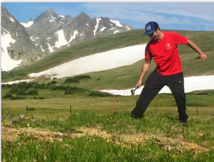
Niwot Ridge: Dylan stakes down rebar to be used as a starting position reference for markers of downslope movement.
