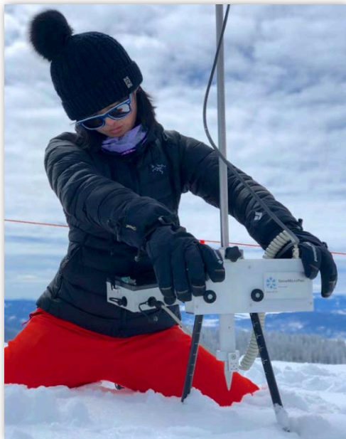
Kehan Yang uses a SnowMicroPen to measure the penetration resistance of snow, which helps us better understand snow formation and remotely-sensed radar measurements of snow. Photo Credit: Melissa Estep
