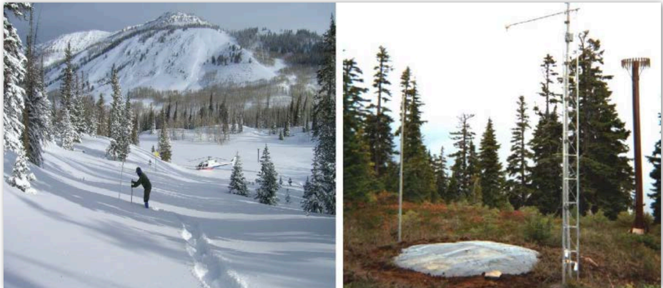
Figure 1. Ground-based snow measurements (left) which cannot be accomplished during COVID-19 due to social distancing requirements and automated Snowpack Telemetry (SNOTEL) sensor (right), which requires ongoing field maintenance also difficult to accomplish during COVID-19. Photo Credit: U.S. Natural Resource Conservation Service (NRCS).
