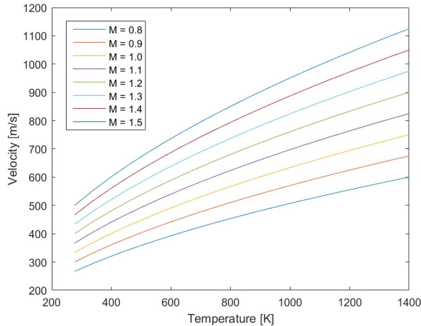
Figure 12. Temperature vs. Velocity at Varying Mach Numbers
