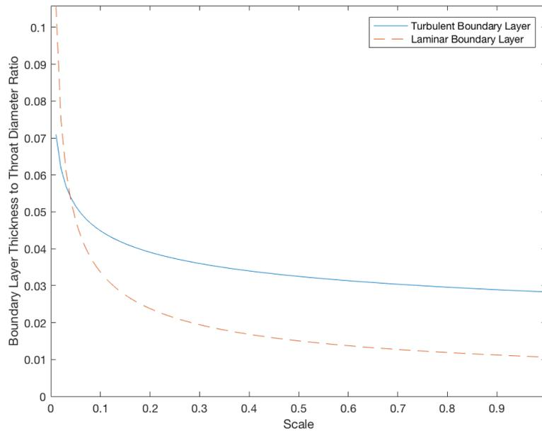
Figure 14. Ratio of Boundary Layer Thickness to Throat Diameter vs. Scale
