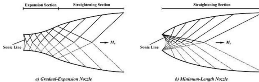
Figure 9. Gradual Expansion Nozzle vs Minimum Length Nozzle
