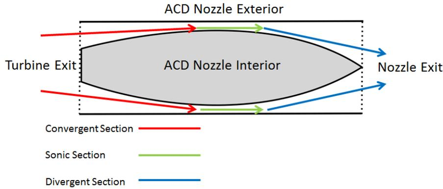
Figure 6. Annular Convergent-Divergent Nozzle Conceptualization
