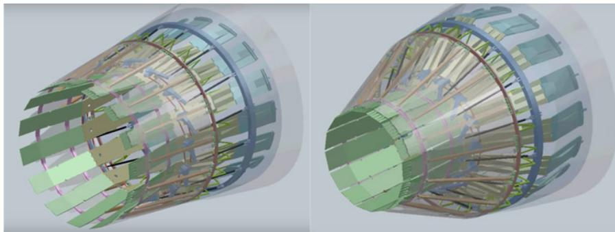
Figure 7. Variable Geometry Nozzle: fully open (left), fully closed (right)
