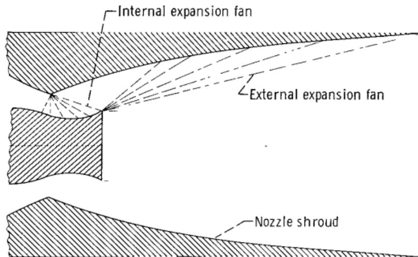
Figure 8. Diagram showing how prandtl-meyer expansion fans accelerate flow in a expansion-deflection nozzle.<sup>6</sup>
