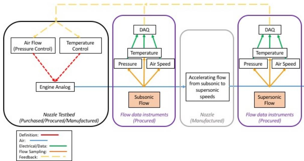
Figure 3. SABRE-Nozzle Functional Block Diagram for Analog Integration
