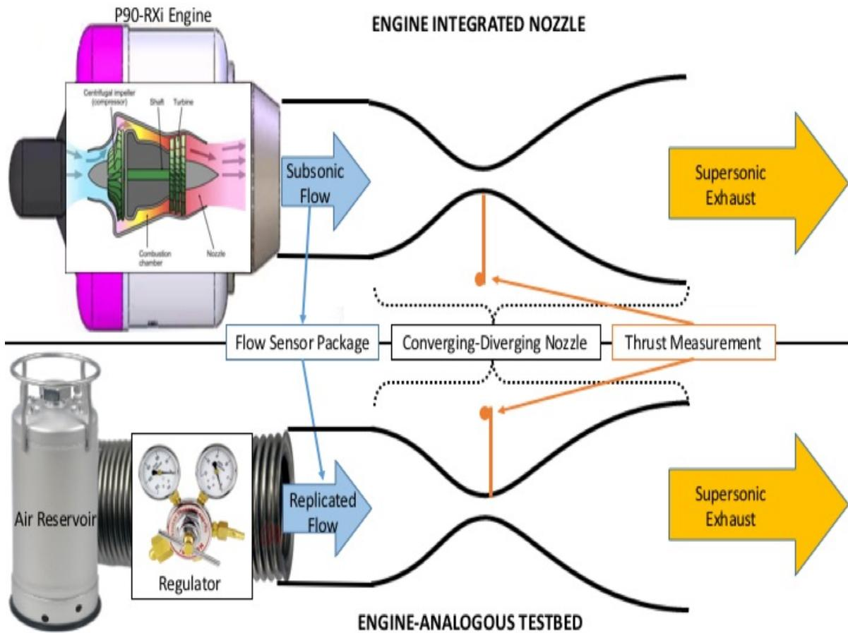
Figure 1. SABRE-Nozzle Concept of Operations
