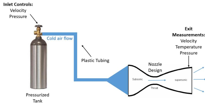
**Figure 11. Cold Flow Testbed Conceptual Diagram**
