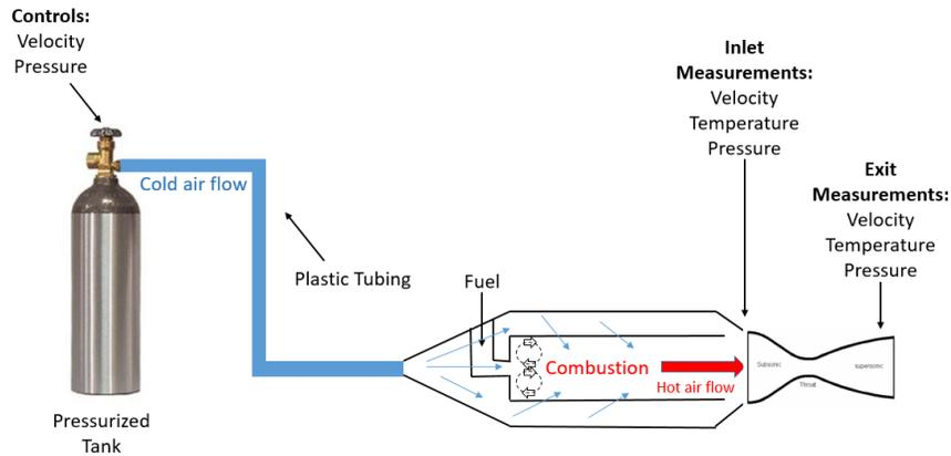
Figure 13. Hot Flow Testbed Conceptual Diagram
