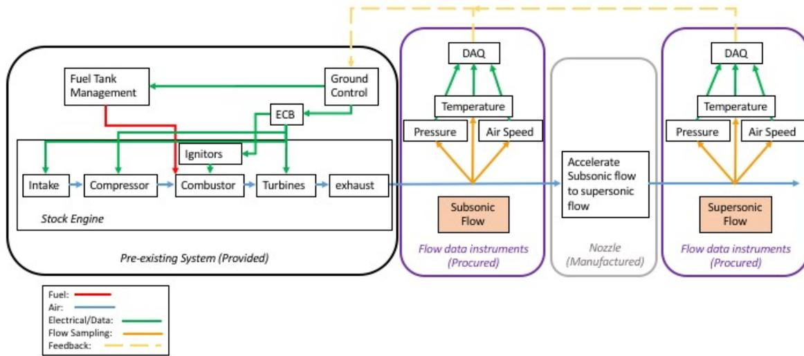
Figure 2. SABRE-Nozzle Functional Block Diagram for Engine Integration
