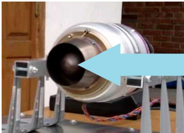
**Figure 18. Dome within nozzle to protect the turbine bearing**
