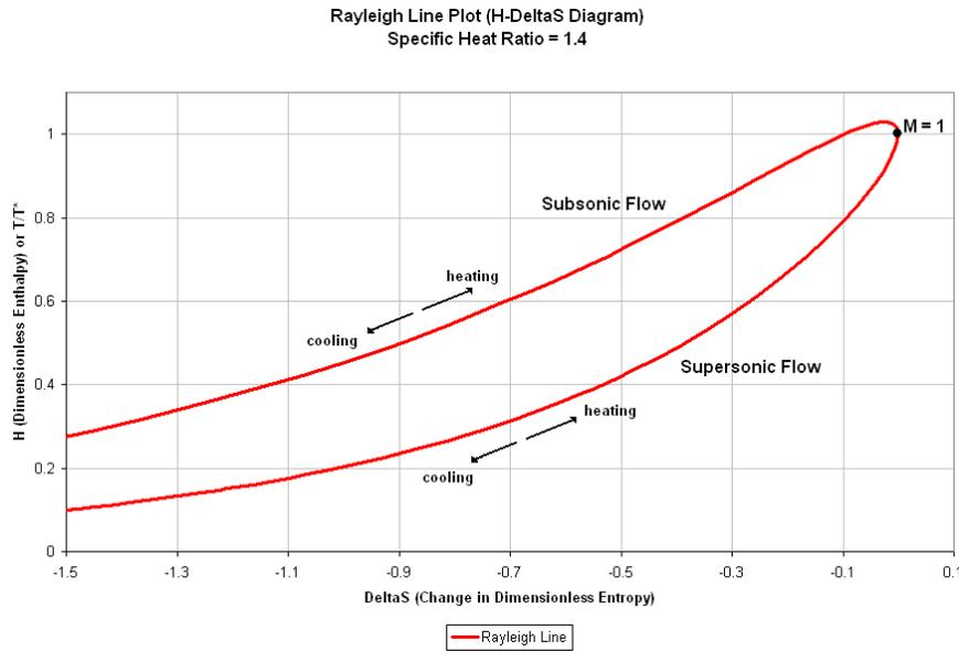
Figure 10. Plot of  $\Delta S$  vs.  $H$  that shows the effects of heating flow.<sup>8</sup>
