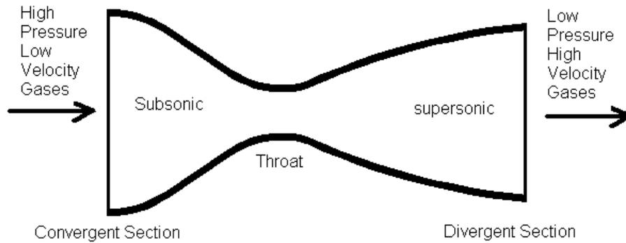
Figure 5. de Laval Nozzle cross-section
