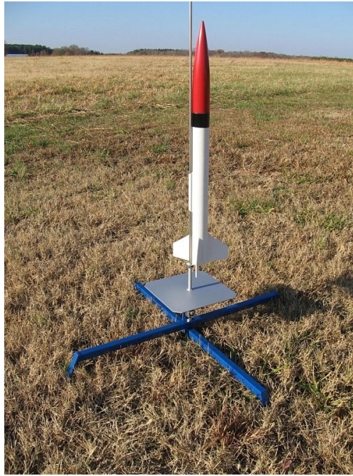
Figure 3.14. Single Fixed Rod Deployment Method 11
