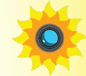
>3D printed aperture casts shadow on photodiodes based on incidence angle
