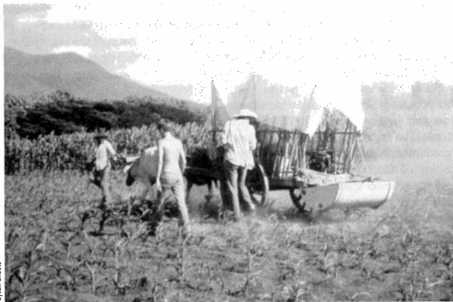
Figure 3-1 Ground-penetrating radar unit collecting data on subsurface stratigraphy. The sending-receiving antenna is attached to the rear of the oxcart. Inside the oxcart are the oscilloscope, instrumentation tape recorder, graphic recorder, gas-powered electric generator, and the geophysicist Hartmut Spetzler. Bill Loker is walking alongside, and Salvador Quintanilla is leading the oxen, named Senate and Cubano, along the grid line.
