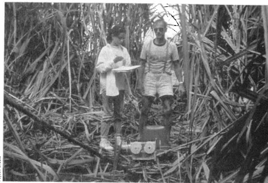
Figure 3-3 Kayla Sheets and Hartmut Spetzler conducting the resistivity survey in a sugar cane field. The instrument at their feet records the resistance of the subsurface to the passage of electricity; rods to their left and right are the electrodes (not visible in this photograph).
