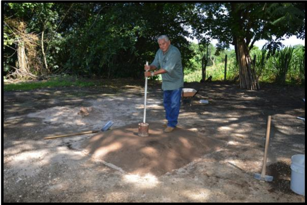
Figure 2-5. The experimental sacbe. Salvador Quintanilla demonstrating the percussive packing device on top of the 2 x 2 meter sacbe replica.
