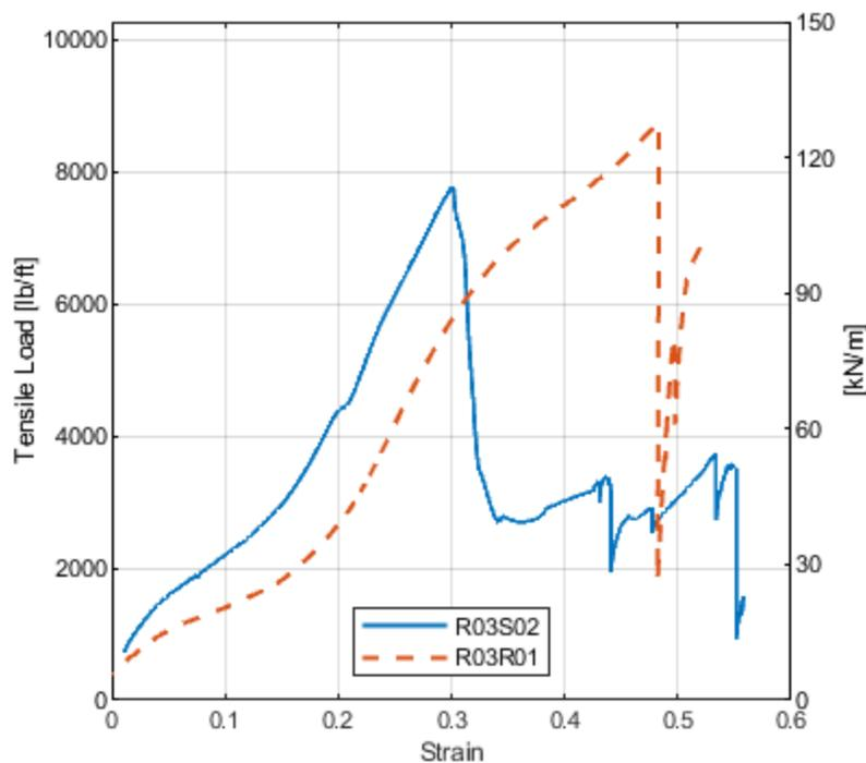
Figure 11. Typical load vs displacement after initial failure (SSM shown)
