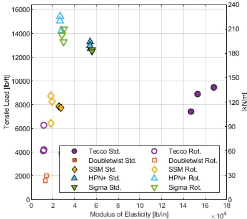
Figure 13. CU Boulder CIEST tension test results
