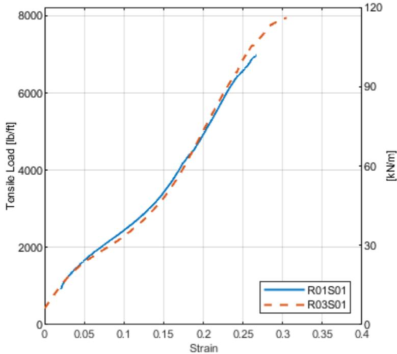
Figure 5. SSM Single Cell Versus Three Cell Testing
