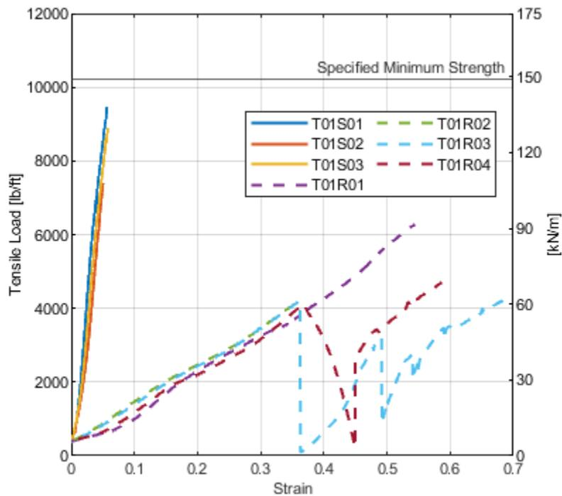
Figure 8. Geobrugg Tecco load vs displacement
