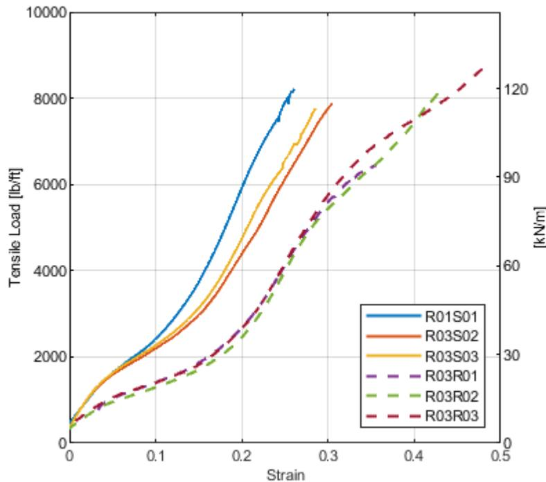
Figure 6. Soil Stabilization Mesh load vs displacement
