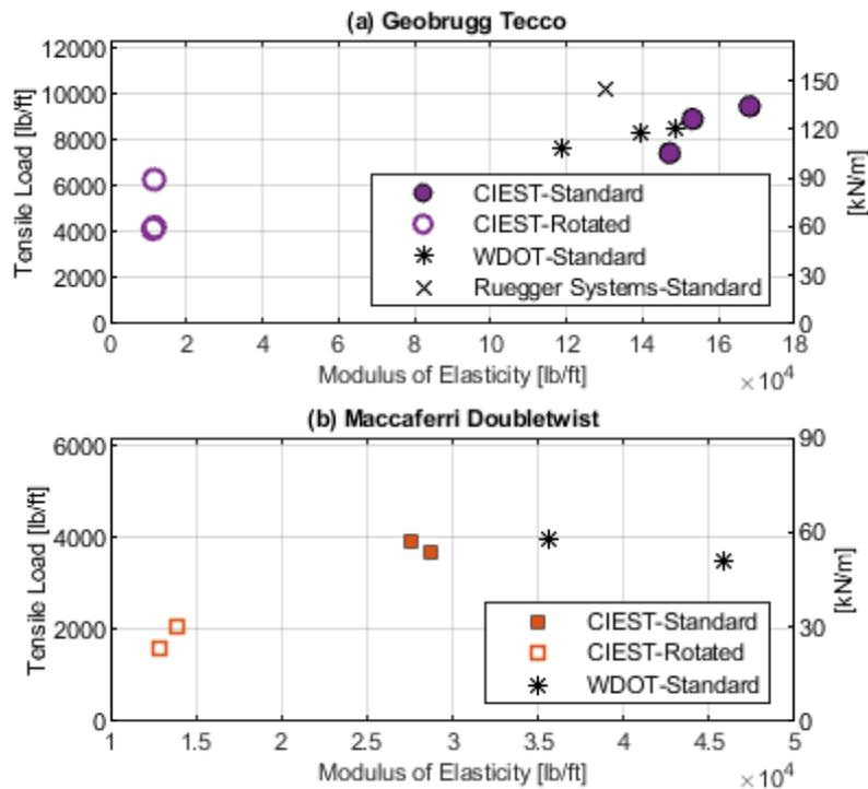
Figure 15. Comparison of tension tests to previous testing results for (a) Geobrugg Tecco and (b) Maccaferri Doubletwist meshes
