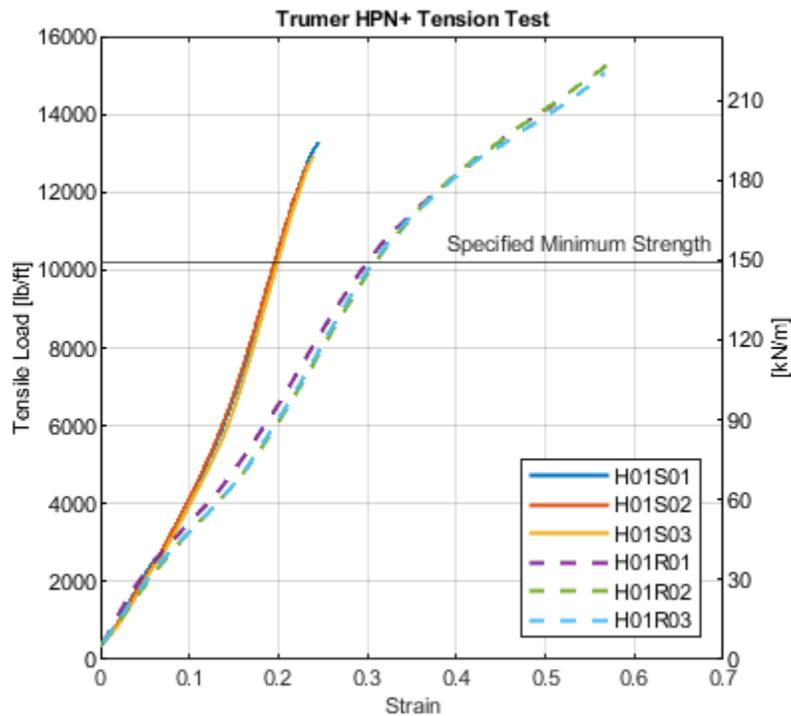
Figure 9. Trumer HPN+ load vs displacement
