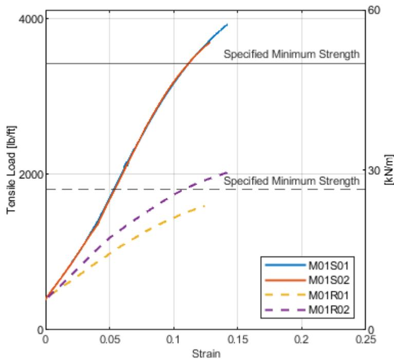
Figure 7. Maccaferri Doubletwist load versus displacement
