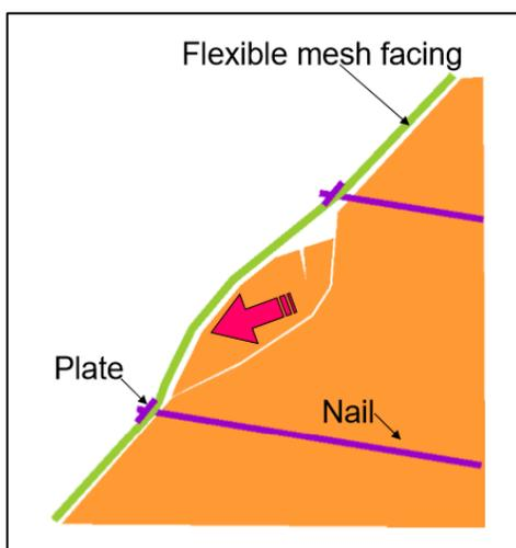
Figure 1. Flexible facing system section view (Maccaferri)
