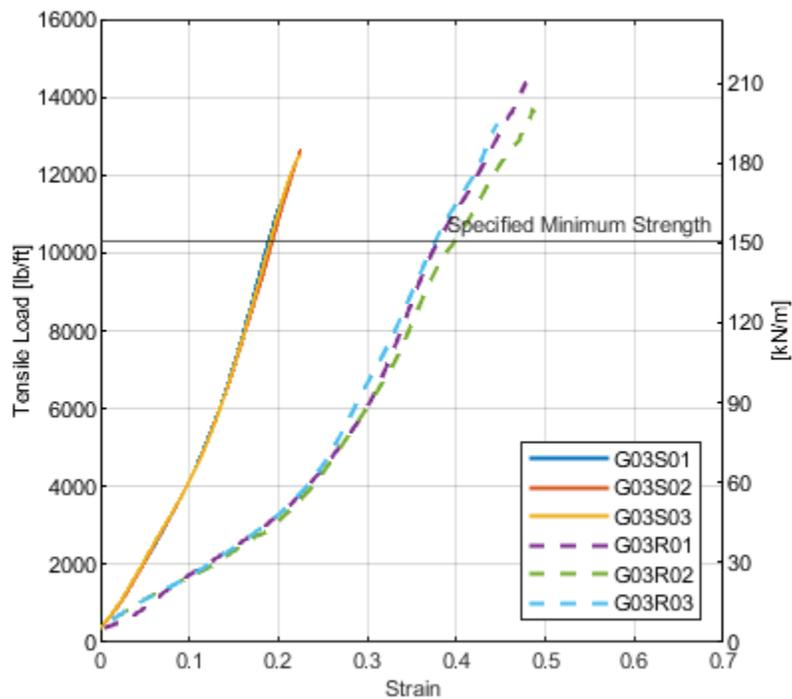
Figure 10. Trumer Sigma load vs displacement
