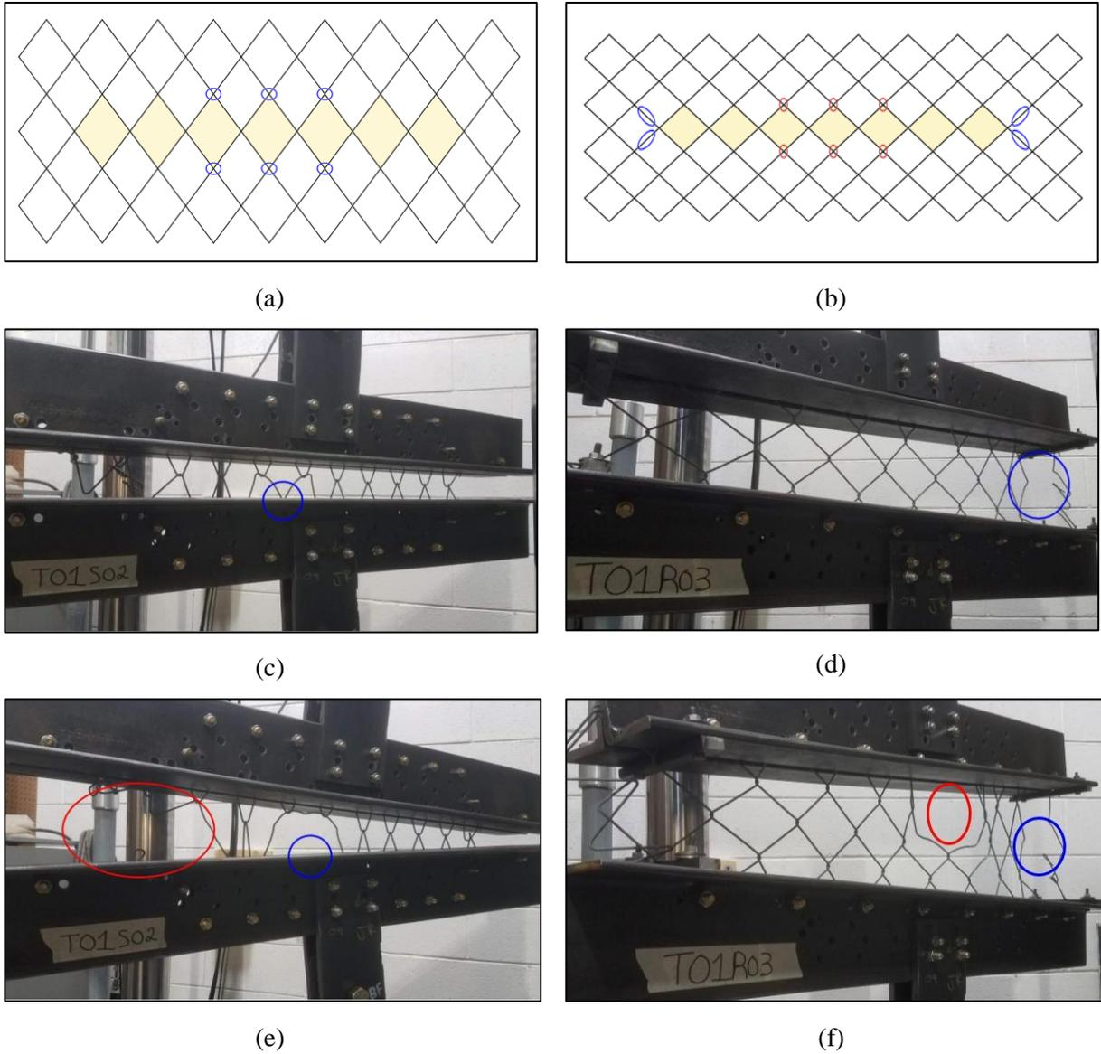
Figure 12. Typical locations of (a) type I and (b) type II failures with initial locations highlighted in blue (c) and (d), and secondary failures highlighted in red (e) and (f).
