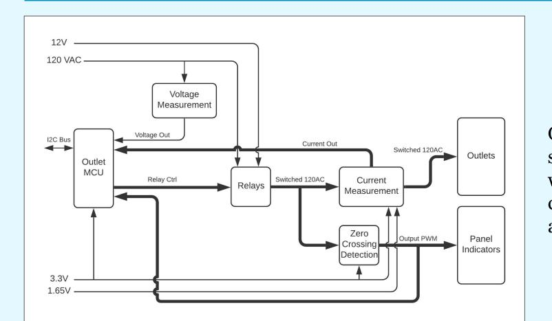
Outlet control and measurement is split into two separate PCBs, one which houses the digital logic (outlet control board), and the other handles all high current devices (relay board).
