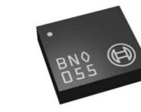
**BNO055** Gyroscope detects the rotation of hand
