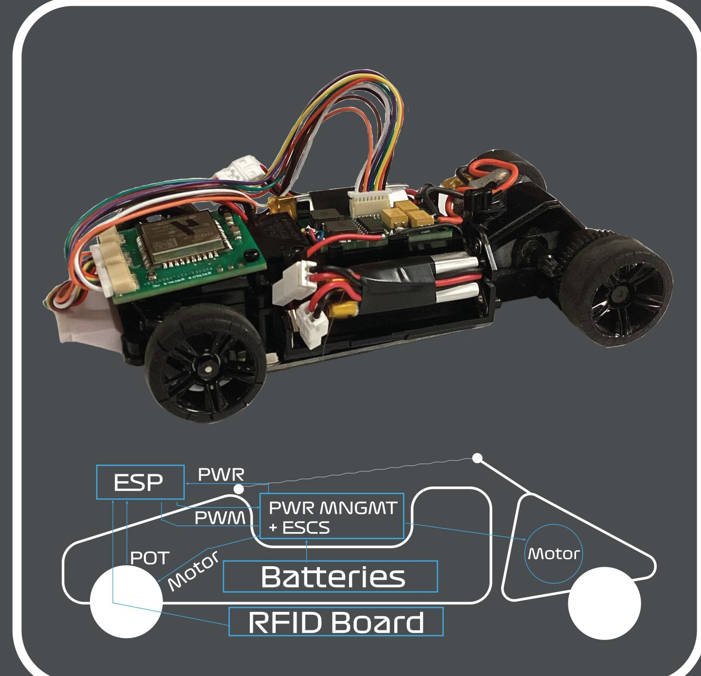
The Formula CU Racing Platform is a is an innovative project that uses high-performance, modified Kyosho Mini-Z RC cars. It features timing, boost, variable speed control, and NFC tag reading through an ESP32 microcontroller and Mifare RC522 RFID board. Through this experience we have created a marketing and educational tool for your sponsor Mission Zero.
