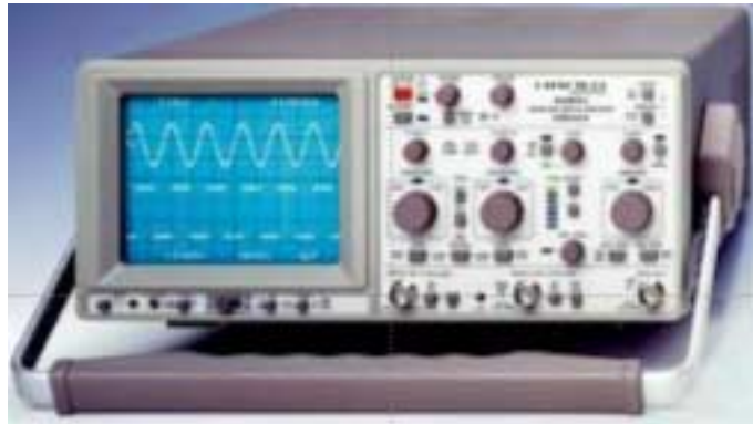
Figure 8.20. This oscilloscope exhibits asymmetric balance due to the extreme screen placement.
