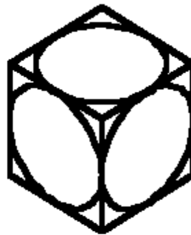
Figure 10.5. Circles appear as ellipses in an isometric drawing.
