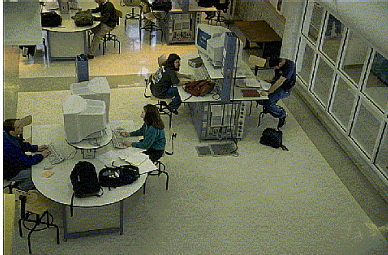
Figure 8.37. Different colors of floor tiles are used in the laboratory plazas to highlight the 20ft x 20ft modular square pattern upon which the ITLL floor plan is based.
