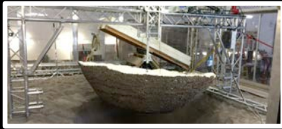
KSC Swamp Works full-scale testing of boulder extraction, 2014
