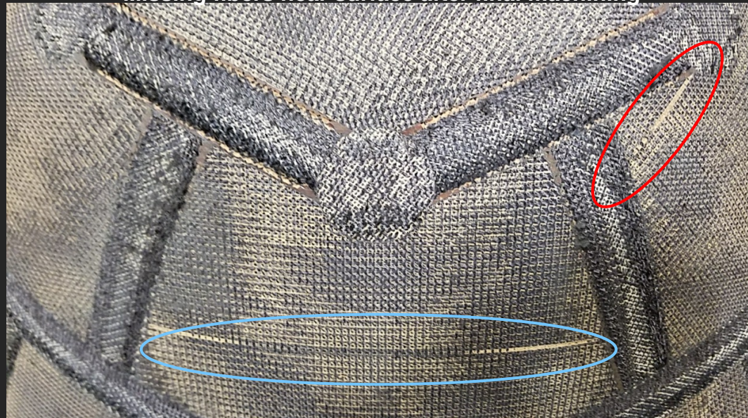
Missing fibers near surface after final machining
