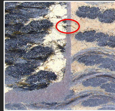
Defect Type: Adhesive Wrinkles and Debonds
