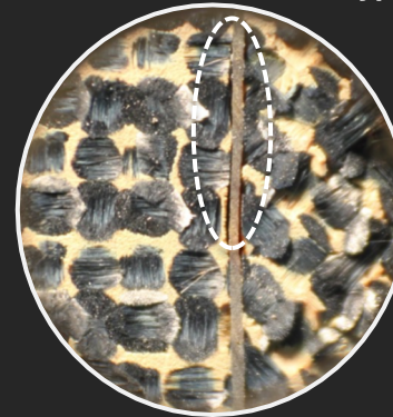
Defect Type: Adhesive Wrinkles and Debonds
