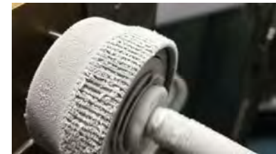
Bulk metallic glass gear testing. Amorphous metal doesn't get brittle in the cold, requires no lubricant.
