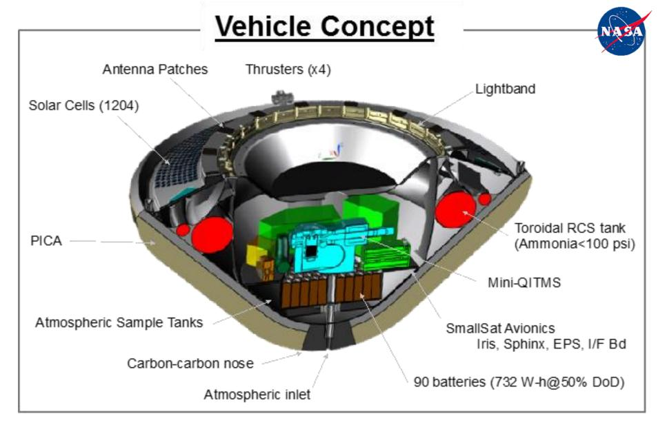
Wet mass is less than 70 kg, including 23% dry mass margins on average
