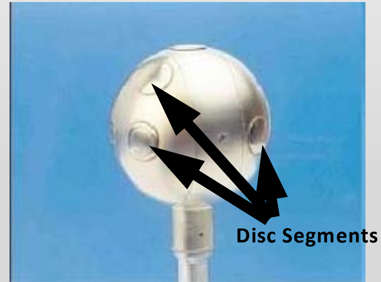
Segmented Langmuir Probes flown on DEMETER [Lebreton et al., 2006]
