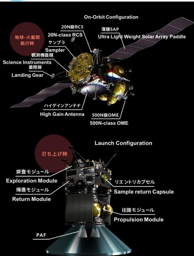
ISAS/JAXA plan to launch the spacecraft in early 2020s. **In order to retrieve the samples,** the spacecraft will need to complete a roundtrip to Mars, circle around the moon and land on its surface.
