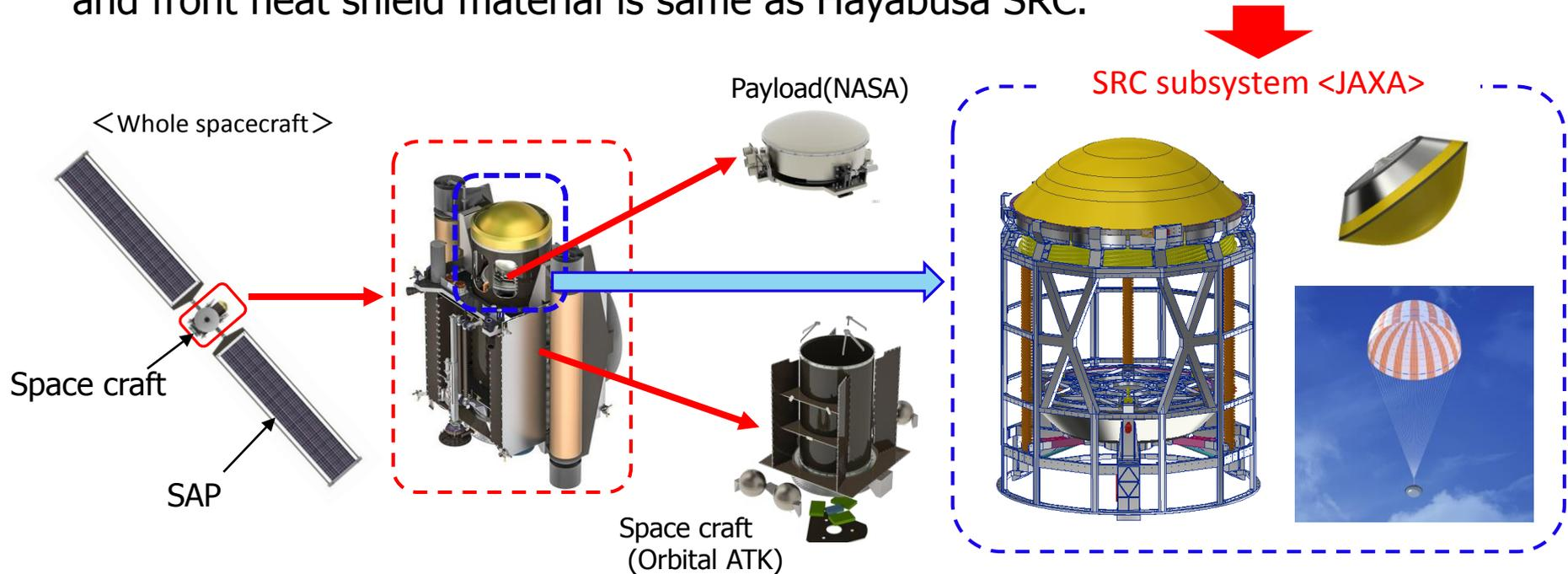
CAESAR-SRC design is modified from HAYABUSA SRC in order to meet the mission requirements of CAESAR. For example, two stage parachute system is adopted to realize a safe deceleration and an integration of onboard devices including the payload system is modified from HAYABUSA SRC to keep samples in low temperature.
