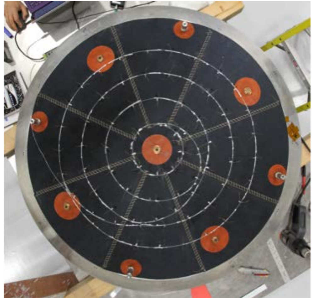
Fiber Optic Strain Sensing Fiber Integrated on EDU Nose in Semi-Spiral Pattern
