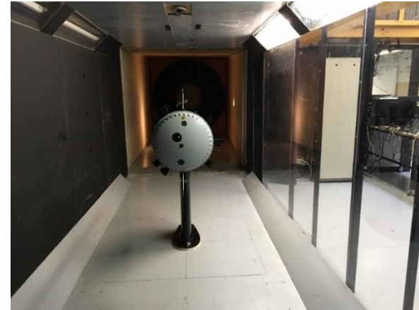
Mock-up mounted on a mast linked to a 6-axis aerodynamic load balance (located under the test section)
