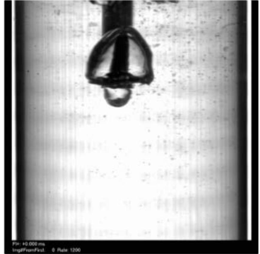
Injector test with chamber at 30 psig
