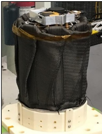
ADEPT SR-1 (4-layer) shown in stowed configuration
