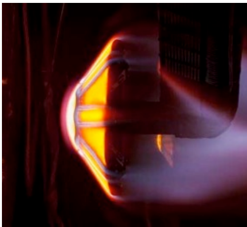
ADEPT SPRITE-C (35cm) tested in Ames IHF arcjet
