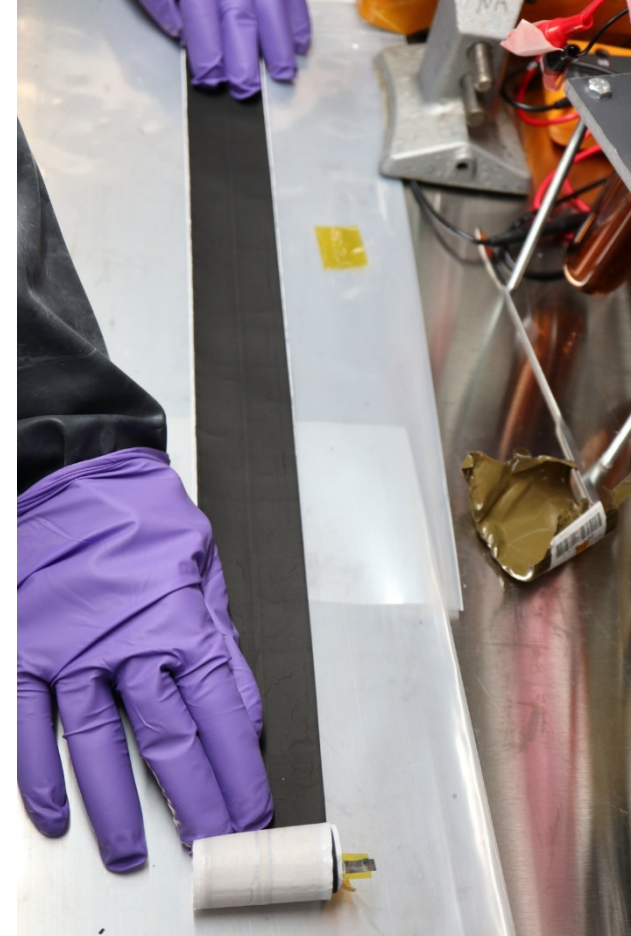
View of cathode and separator, as jellyroll is unwound during DPA
