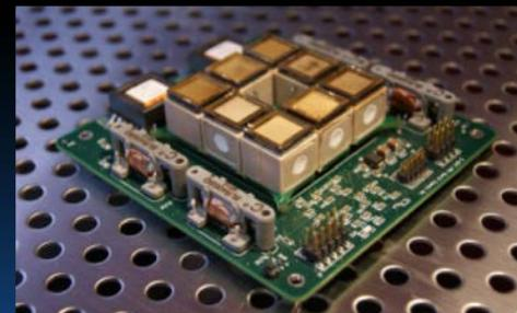
Figure 4.13: S-iEPS propulsion system. Image Courtesy of MIT SPL.
