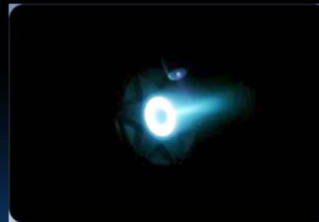
Figure 4.18: BHT-200 during operation. Image Courtesy of Busek Co Inc.
