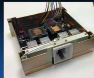
Figure 4.16: PPTCUP propulsion system.
