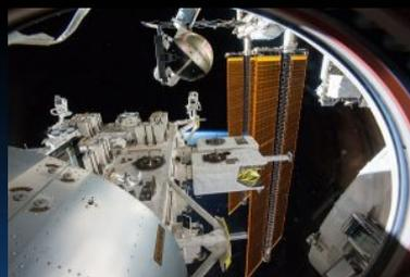
Figure 4.9: SpinSat Mission deploying from International Space Station
