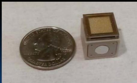
Figure 4.12: Electropray thruster. Image Courtesy of MIT SPL.
