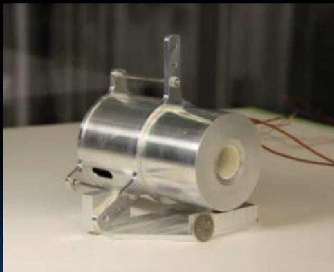
Figure 4.19: Cylindrical Hall Effect Thruster. Image Courtesy of UTIAS SFL.
