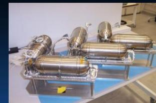
Figure 4.6: SSTL butane propulsion system. Image Courtesy of Gibbon (2010).
