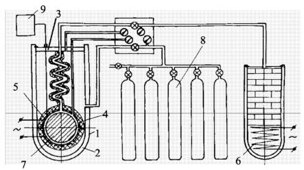
Early Veneras (4-8) had 'cold' structure, with external insulation. Insulation performance depends on gas, so CO2 at high pressure was used in some tests on fullscale vehicle.
