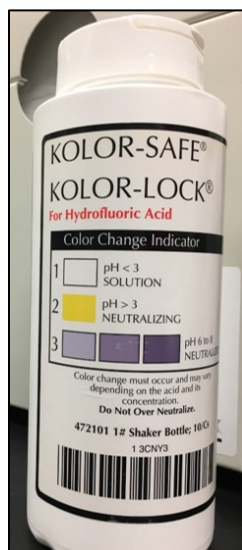
Figure 8.4 Kolor-Safe® / Kolor-Lock® Solidifier for hydrofluoric acid neutralization
