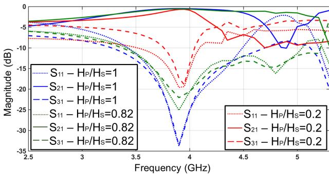
Fig. 3. Electromagnetically-simulated response in terms of S-parameters for alternative levels of  $H_p/H_s$ . The circulator dimensions are identical for both designs. The DC magnetic bias field is altered as shown in Fig. 4.
