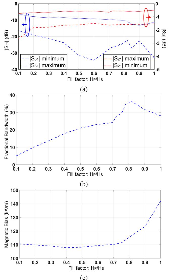
Fig. 4. Circulator performance for alternative levels of  $H_p/H_s$ . (a) Power transmission response:  $S_{21}$ ,  $S_{31}$ , (b) FBW, and (c) DC magnetic bias.
