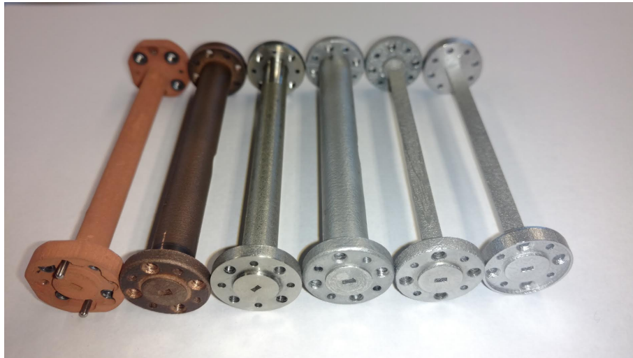
Figure 6.3: Straight 10 cm WR-10 waveguides implemented in a variety of materials. From left to right: metal (Cu) coated plastic (MCP), GRCoP-84 (Cu), Inconel 625 (Ni), and 3 AlSi10Mg with different laser settings.
