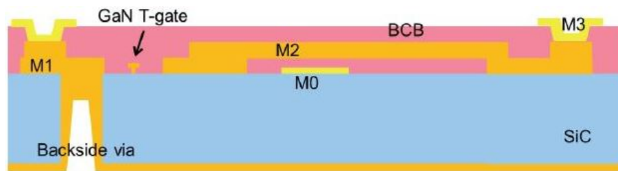
Figure 4.2: Cross-section view of CMP Cu interconnects combined with GaN-on-SiC MMIC technology. Source: [4]
