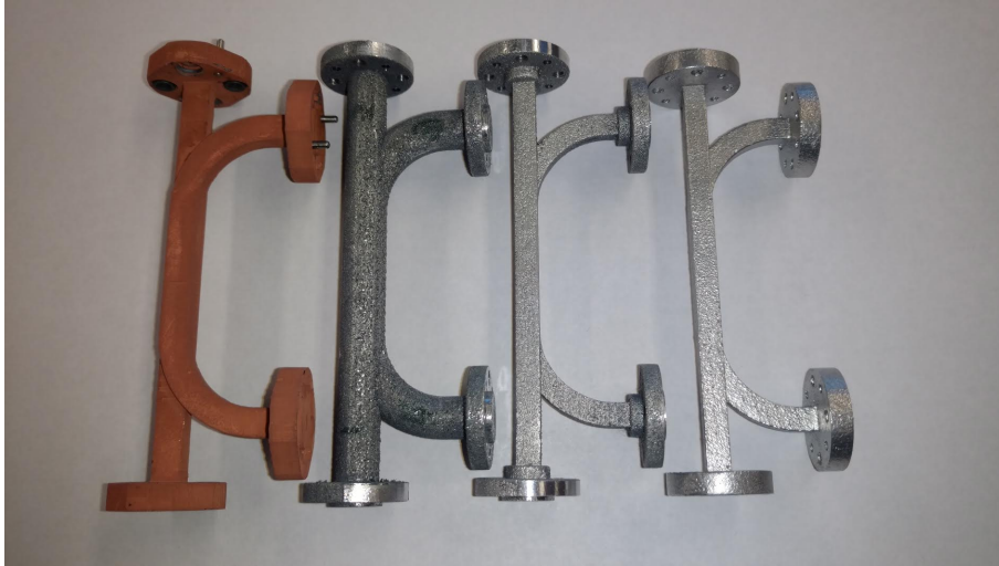
Figure 6.4: From left to right: WR-10 20 dB directional couplers in metal (Cu) coated plastic (MCP) and AlSi10Mg with different laser settings.
