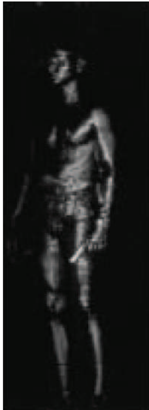
Figure 1.4: Image from an active f = (27\text{--}33) GHz holographic imaging system, developed at PNNL. The test subject is a mannequin with concealed objects beneath its clothing, and a weapon in its hand. Image taken from [25].
