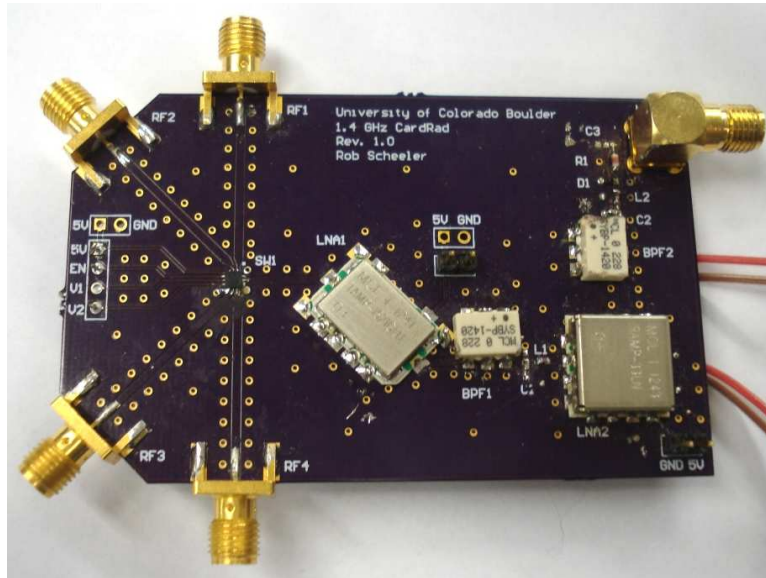
Figure 6.2: Example PCB of a radiometer integrated on a single board.
