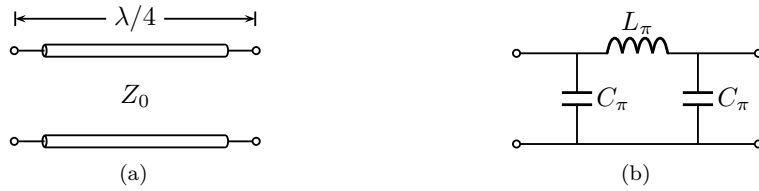
Figure 3.7: A quarter wavelength transmission line (a) and the lumped element \pi equivalent circuit (b).
