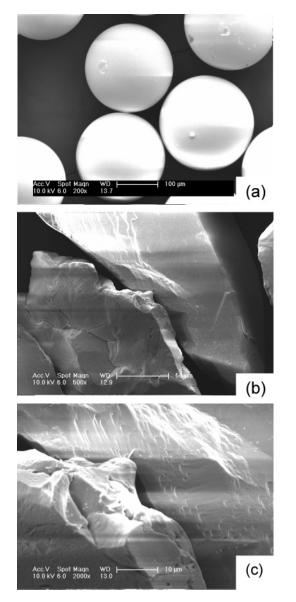
FIGURE 6. ESEM images of (a) spherical glass bead collectors (200× magnification, 100  $\mu$ m bar) and irregularly shaped quartz grains at (b) 500× magnification (50  $\mu$ m bar) and (c) 2000× magnification (10  $\mu$ m bar).
