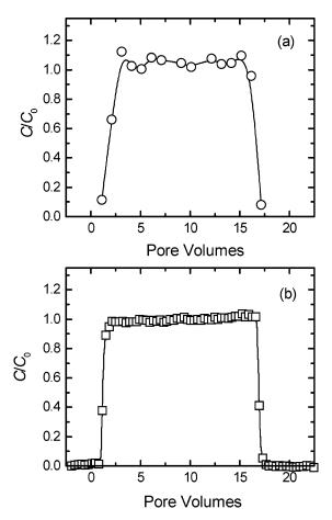
FIGURE 7. Breakthrough curves for experiments conducted in columns packed with soda-lime glass beads with (a) *C. parvum* oocysts and (b) 4.1  $\mu$ m model latex particles suspended in DI water. Other experimental conditions were as follows: approach velocity = 0.042 cm/s, porosity = 0.36, mean bead diameter = 0.23 mm, unadjusted pH (varied between 5.6 and 7.1), and temperature = 22–23 °C.
