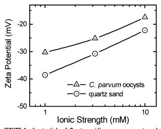
FIGURE 1.  $\zeta$  potentials of *Cryptosporidium parvum* oocysts and clean quartz grains as a function of ionic strength at unadjusted pH of 5.6–5.8.
