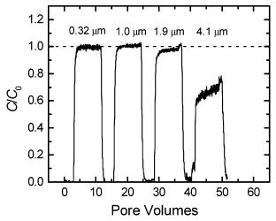
FIGURE 8. Breakthrough curves for experiments conducted with model latex particles of increasing diameter (0.32, 1.0, 1.9, and 4.1  $\mu$ m) suspended in DI water in a column packed with clean quartz sand. Other experimental conditions include approach velocity = 0.042 cm/s, porosity = 0.43, mean grain diameter = 0.21 mm, pH 5.6-5.8, and temperature = 22-23 °C.
