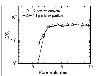
FIGURE 4. Breakthrough curves for experiments conducted with *C. parvum* oocysts and 4.1  $\mu$ m model latex particles in columns packed with clean quartz sand at 1 mM ionic strength. Other experimental conditions include approach velocity = 0.042 cm/s, porosity = 0.43, mean grain diameter = 0.21 mm, pH 5.6–5.8, and temperature = 22–23 °C.
