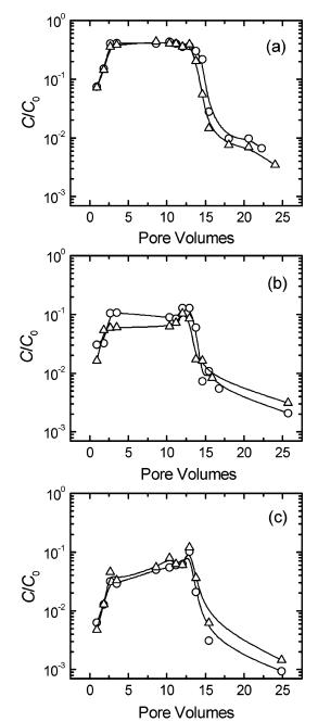
FIGURE 2. Breakthrough curves for two replicate experiments conducted with *C. parvum* oocysts in columns packed with clean quartz grains at three different solution ionic strengths: (a) 1 mM KCI; (b) 3.16 mM KCI; and (c) 10 mM KCI. Other experimental conditions were as follows: approach velocity = 0.042 cm/s, porosity = 0.43, mean grain diameter = 0.21 mm, pH 5.6–5.8, and temperature = 22-23 °C.
