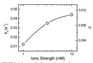
FIGURE 3. Influence of ionic strength on the *C. parvum* oocyst deposition rate coefficient ( $k_d$ ) and the corresponding singlecollector removal efficiency ( $\eta$ ) in a column packed with quartz sand. Each data point represents the average value determined from all experiments conducted at a given ionic strength. Oocyst deposition rate coefficients were calculated using breakthrough concentrations ( $C/C_0$ ) in Figure 2 and eq 1.
