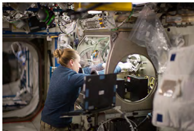
NASA astronaut Kate Rubins during setup of the SODI instrument with the DCMIX3 cell array in the microgravity glovebox MSG (NASA image).
