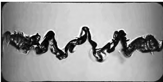
Figure 2: Interfacial patterns in miscible liquids under vibrations parallel to initially horizontal interface at f=8\text{Hz} , A=10.7\text{mm} . (left: on ground; right: in microgravity)
