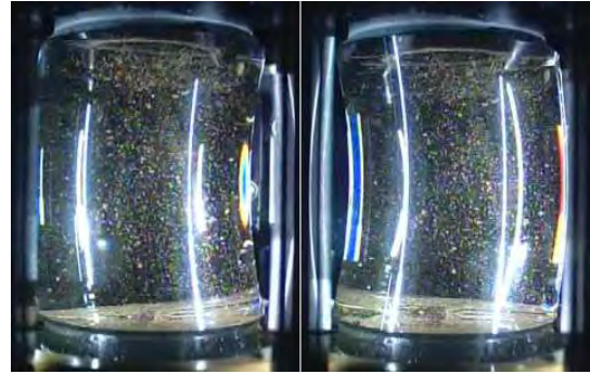
Figure 6: Images of the liquid bridge oscillation the experiment Dynamic Surf . The images were kindly provided by Dr. Satoshi Matsumoto.
