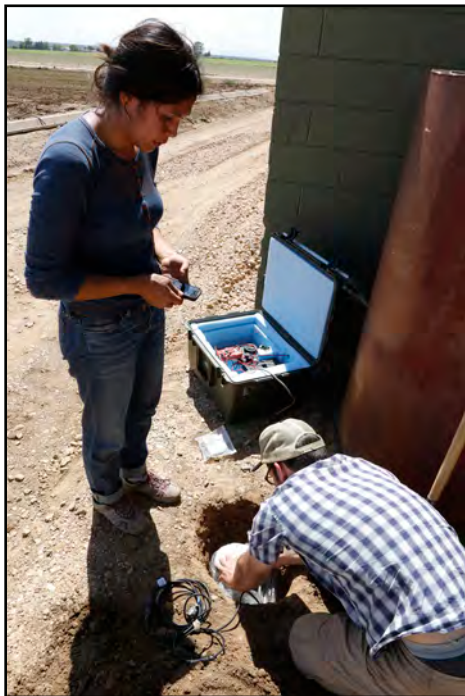
CU geology graduate students William Yeck, Matthew Weingarten, and Jenny Nakai deploying seismometers
