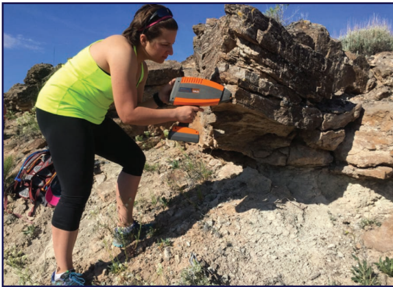
Geology graduate student Sarah Black, human rover, collecting VNIR hyperspectral data of a Jurassic microbialite.
