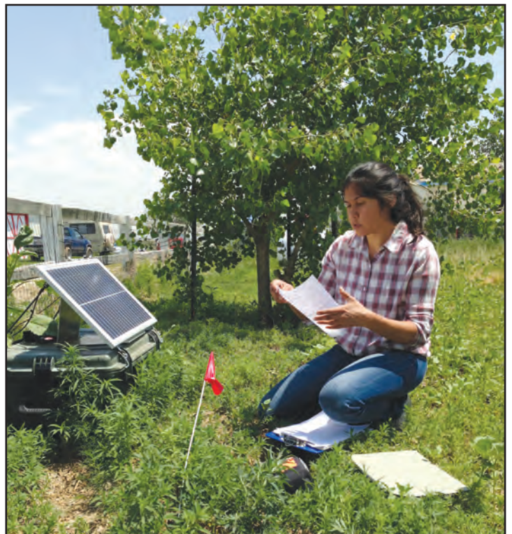
Jenny Nakai (PhD '18) downloading data from seismograph station near Greeley, Colorado.
