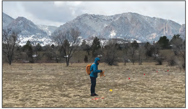
Undergraduate Corey Flynn sets up magnetics and ground conductivity survey for field geophysics class, CU South Campus.
