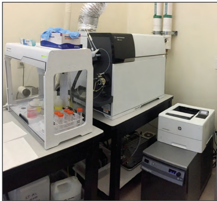
Agilent 7900 quadrupole ICPMS
