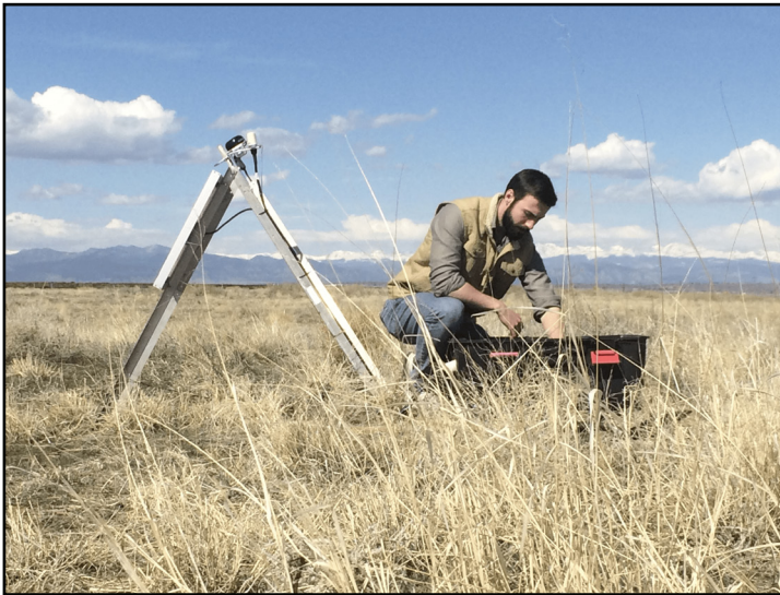
Graduate student Tom Clifford performs maintenance on earthquake seismic station at Rocky Mountain Arsenal, Colorado. photo credit: Anne Sheehan
