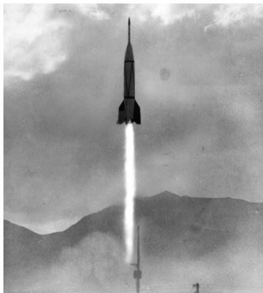
Figure 1.1: The two-stage Bumper rocket with a combination of a V-2 and WAC Corporal, launching into the hypersonic regime on February 24th, 1949. Image from the National Air and Space Museum [6].
