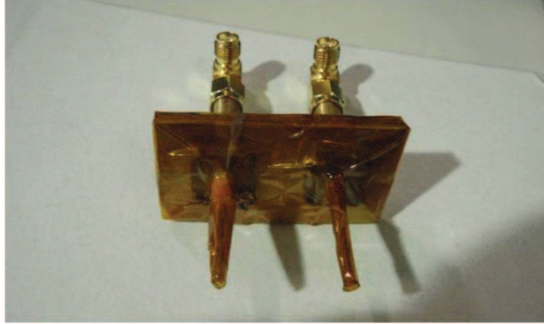
Figure 5.5: RF transmission probe for plasma density measurement (Courtesy of EDA)
