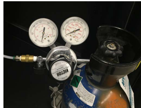
CO 2 cylinder – When on, flow should be between 14.5 psi and 21.7 psi
