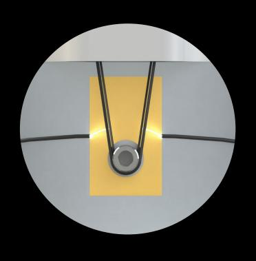
Electronics send current through highly resistive wire to burn through restraint lines initiating deployment
