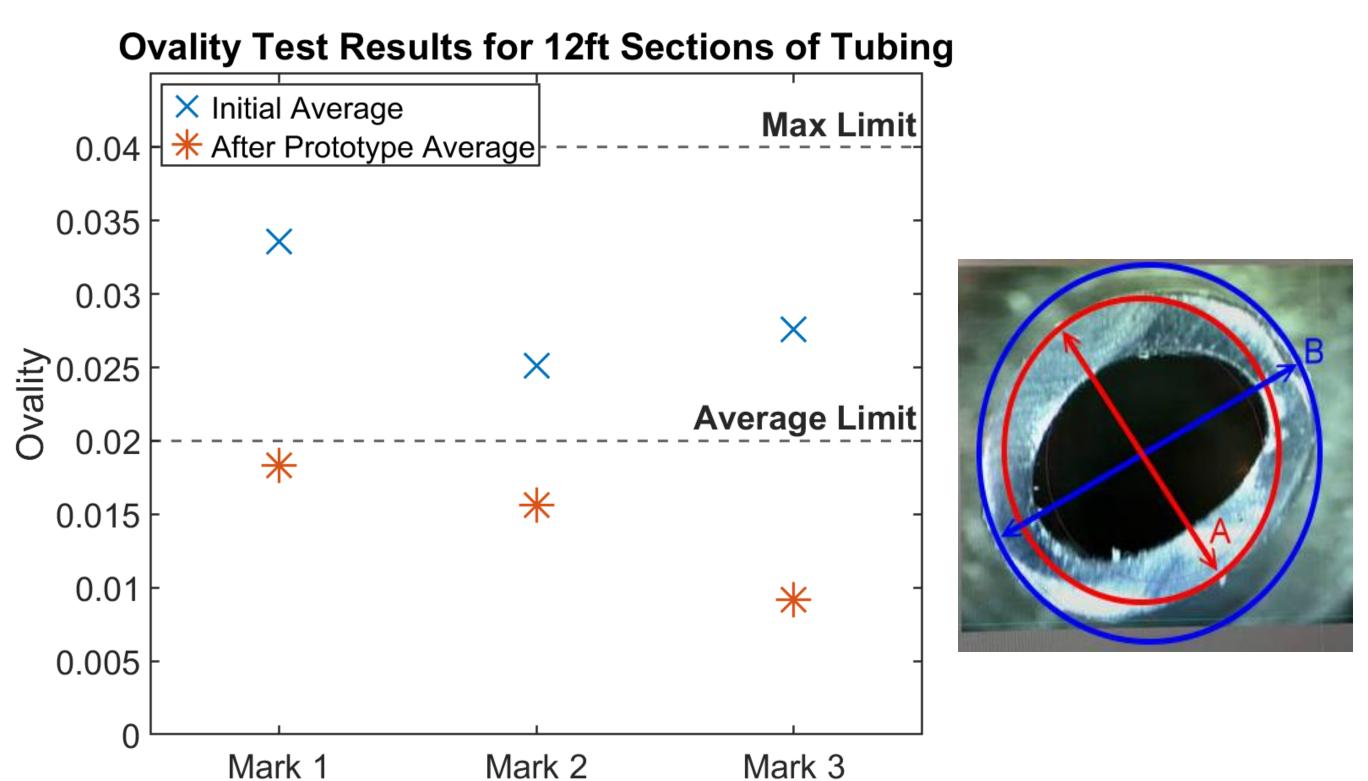
After heating and reforming the tubing, we observed significant improvement in ovality, rendering more of the tubing within spec.
