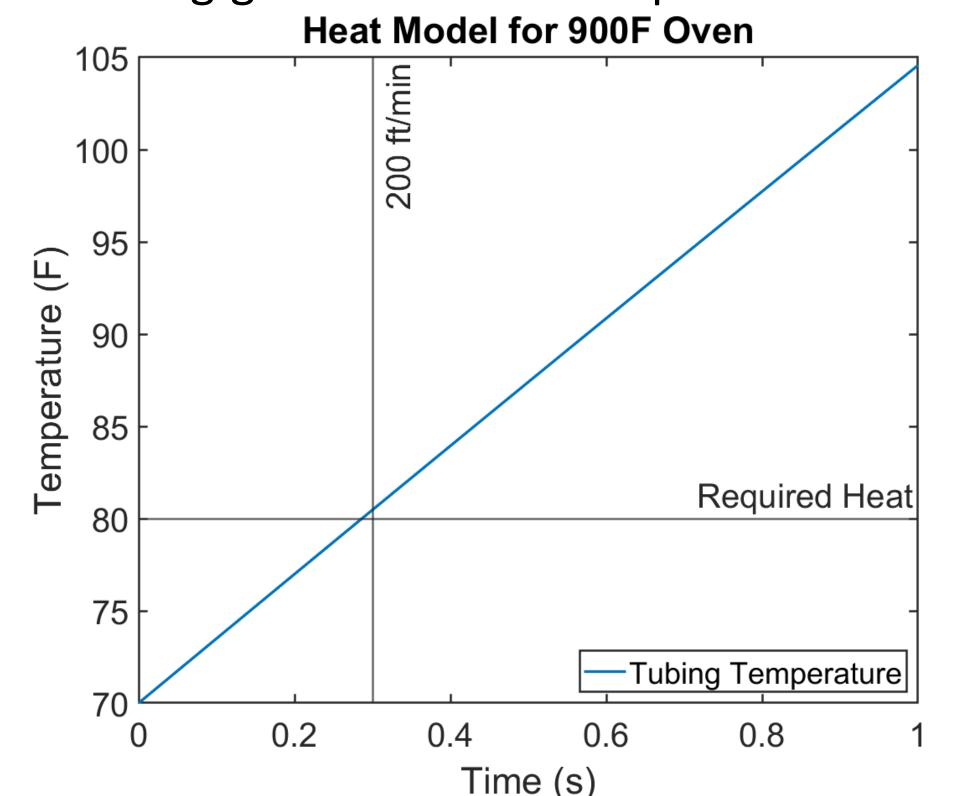
Differential Equation Governing Tubing Temperature  $\frac{\sigma dC_P}{4} \left(\frac{dT}{dt}\right) = h(T_{\infty} - T(t)) + \sigma \varepsilon_{tubing}(T_S^4 - T(t)^4)$  Assembly
