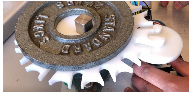
Geneva wheel with 2.5-lb additional load
