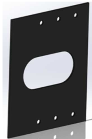
Figure 8: A sealing gasket located between the disc housing and the expansion tank
