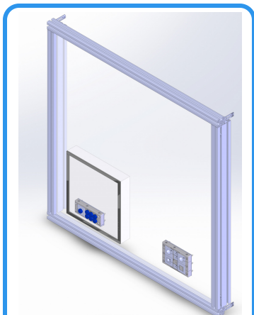
The back subassembly of the chamber showing sealing and accessibility features.
