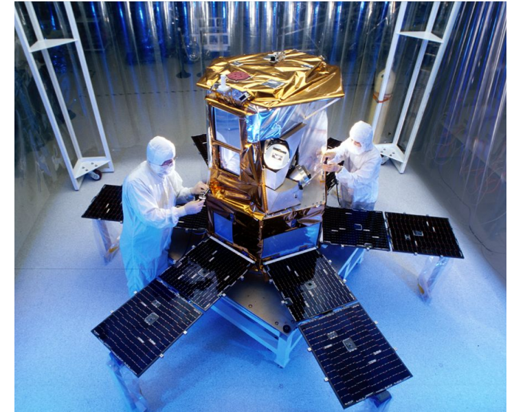
Solar Radiation and Climate Experiment (SORCE) Satellite in a LASP clean room
