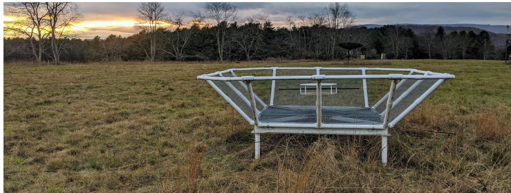
Figure 4: Deployed PAPER antenna at Green Bank WV, set-up for zenith pointed drift scans.
