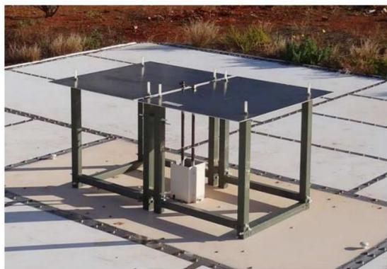
Figure 1: Photograph of the EDGES high band blade dipole antenna placed over the ground plane.
