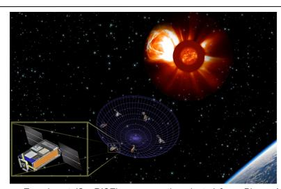
The Sun Radio Interferometer Space Experiment (SunRISE) was recently selected for a Phase A study as a Heliophysics Explorer Mission of Opportunity. Consisting of six small spacecraft spread over 10 km slightly above geosynchronous orbit, SunRISE will image bright solar radio bursts to track the origin and transport of solar energetic particles. NESS Co-I Kasper is the PI of SunRISE.
