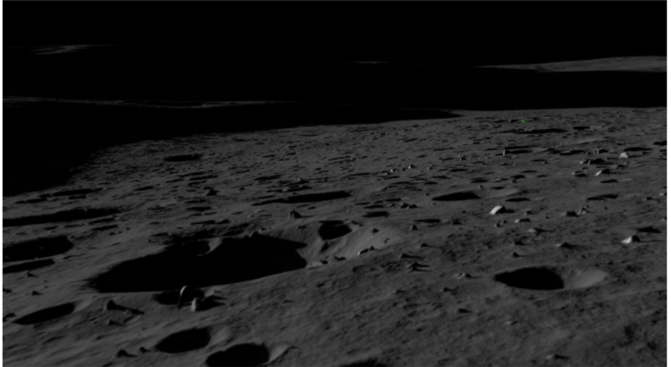
Figure 2: Synthetic lunar digital elevation model of the terrain near Hermite A. The model has a resolution of approximately 4 cm/pixel (grid posting).
