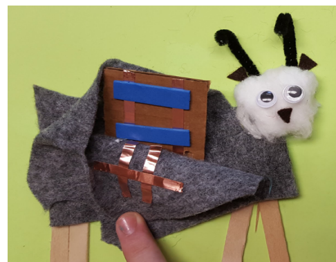
Figure 2: Copper tape button embedded in a crafted goat from a "Busy Spider" tactile page.
